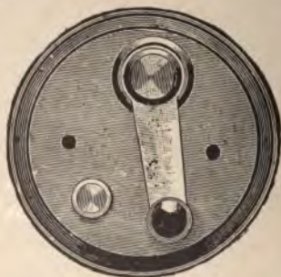
FIG. 132.—Ordinary two-point lever switch of the type used in connection with switchboard night alarm circuits, as shown in Fig. 107.
